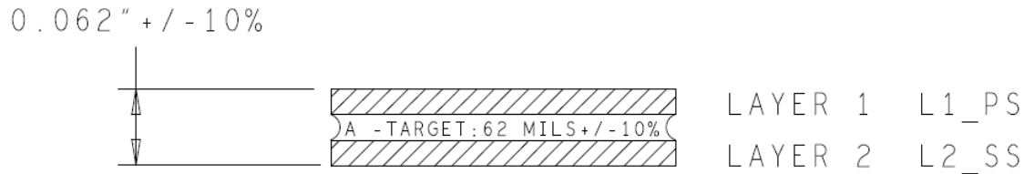
Figure 17. FRDM-CR20A PCB stackup cross-section (four layer)
