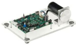
MTRCKTSBNZVM128 3-phase BLDC Motor control kit
