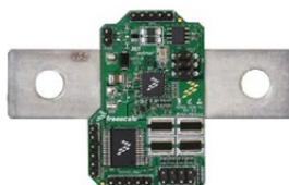
RD9Z1-638-4Li 14.4 V battery monitoring MM912J638 reference design
