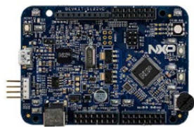
DEVKIT-S12ZVC CAN node S12ZVC192 evaluation board
