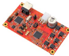
S12ZVML-MINIXXX 3-phase PMSM Motor control kit
