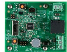
S12VR32EVB Relay-based DC S12VR32 evaluation board
