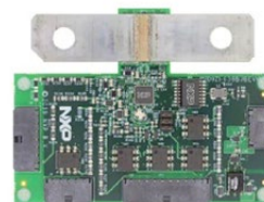
RD9Z1-638BJBEVM Battery junction box MM912J638 reference design
