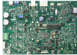
S12ZVMC256EVB 3-phase BLDC and PMSMS12ZVMC256 evaluation board
