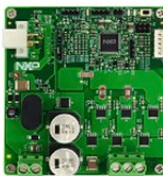
S12ZVM-EFP Electrical Fuel Pump S12ZVML128 reference design
