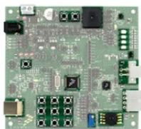
VLG-MC9S12ZVC CAN node S12ZVC192 evaluation board
