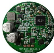
S12ZVM-EWP Electrical Water Pump S12ZVML64 reference design
