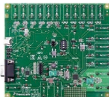
KIT9Z1J638EVM battery monitoring MM912J638 evaluation board
