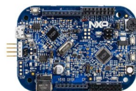
DEVKIT-S12ZVL LIN node S12ZVL32 evaluation board
