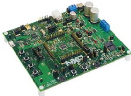
S12ZVMBEVB Reversible DC S12ZVMB evaluation board
