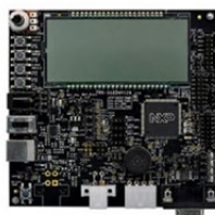
TRK-S12ZVH128 Instrument cluster S12ZVH128 evaluation board
