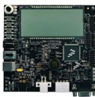
TRK-S12ZVHY64 Instrument cluster S12ZVHY64 evaluation board
