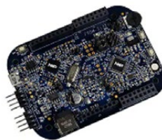
DEVKIT-ZVL128 LIN node S12ZVL128 evaluation board
