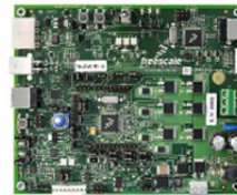
S12ZVMEVB 3-phase BLDC and PMSM S12ZVM(L/C)128 evaluation board
