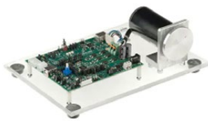
MTRCKTSPNZVM128 3-phase PMSM Motor control kit
