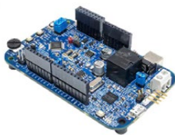
DEVKIT-S12VRP Relay-based DC S12VRP64 evaluation board
