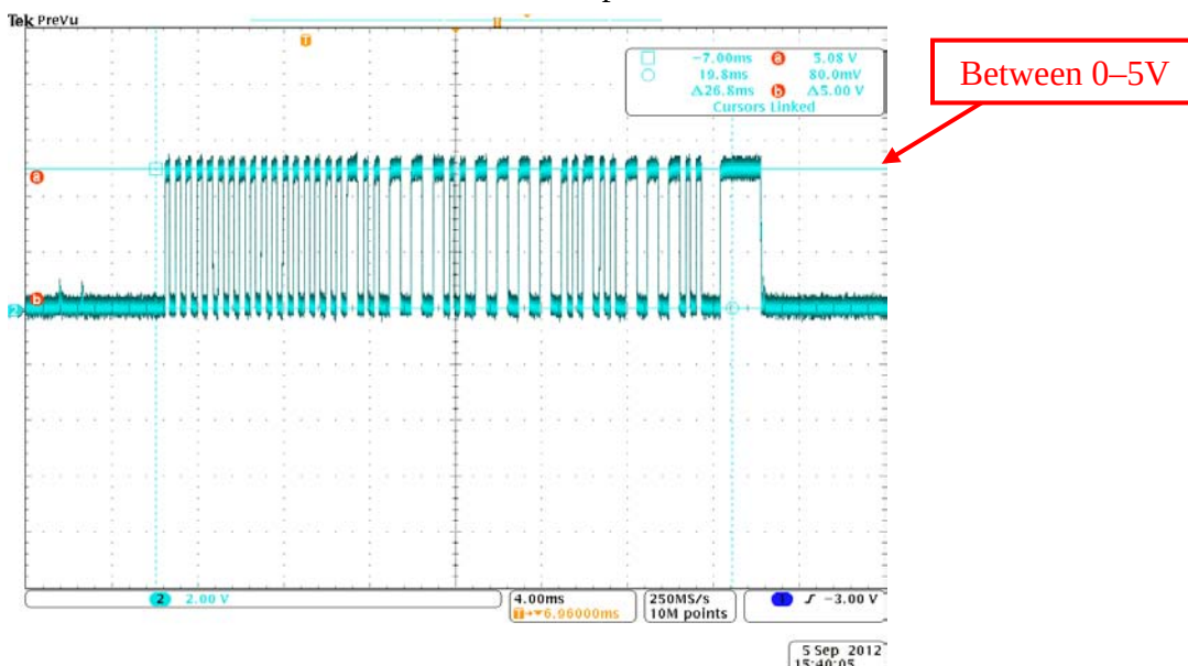
Figure 15. Communication wave after the comparator circuit
