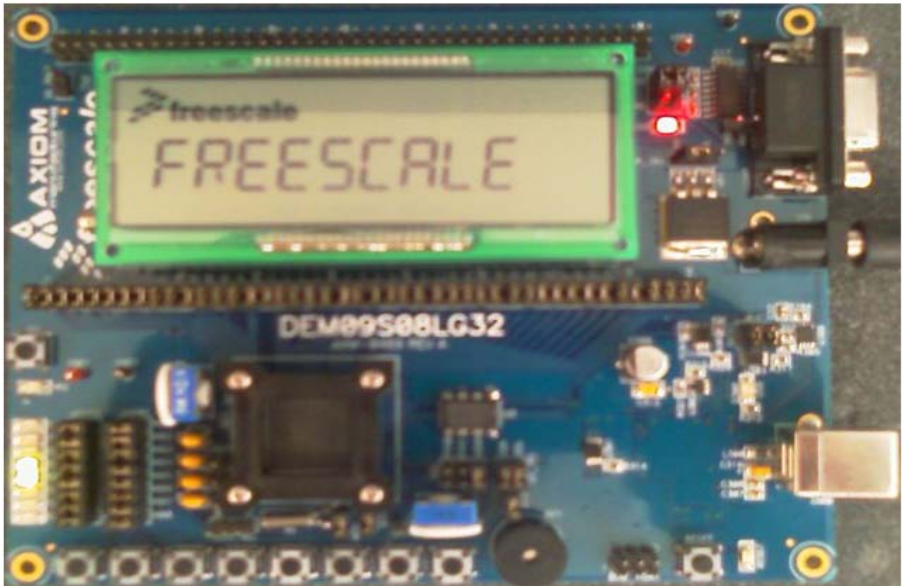
Figure 1. MC9S08LG32 Demo Board LCD Setup
