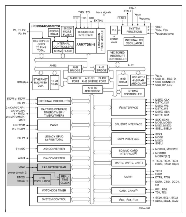
View additional information for Arm7<sup>™</sup> with 128 kB flash, 34 kB SRAM, Ethernet, USB 2.0 Device, CAN, and 10-bit ADC.
